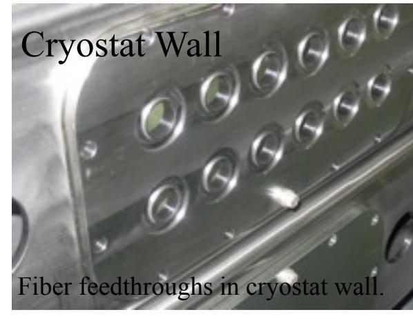
Fiber feedthroughs in cryostat wall.
