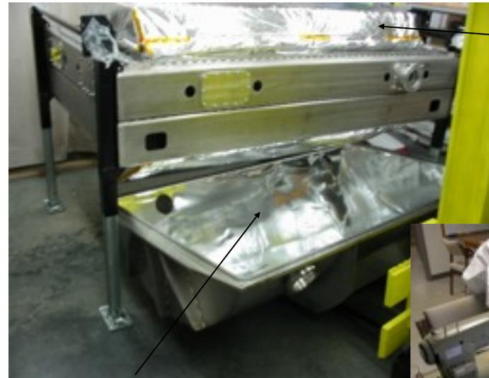
Aluminized mylar sheets on inner-surface of warm vessel walls.
